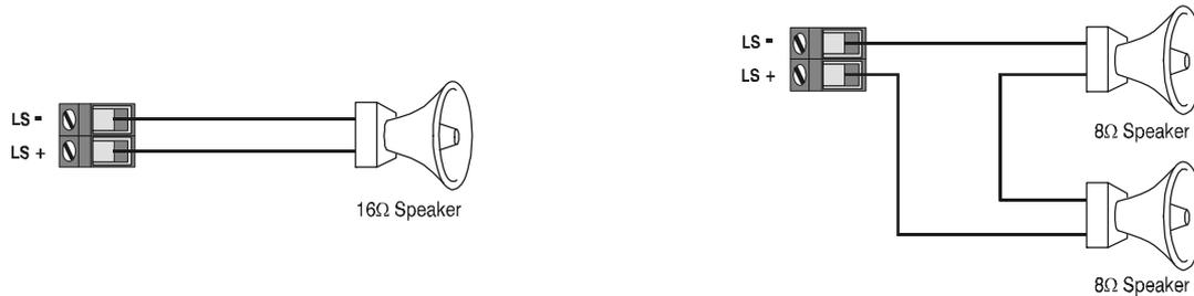
**NOTE** The total load including the built-in speaker must not be less than 16Ω (e.g. 1 x 16Ω speaker, 2 x 8Ω speakers in series, etc.).
