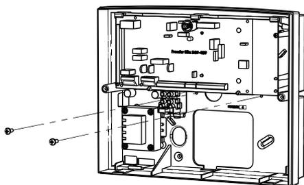
**Step 2: Fit battery into place, position the clamps against the top face of the battery and tighten screws.**
