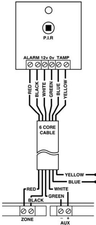
Figure 2a - Wiring a Single Powered Detector to a Zone (see also Figure 4).
