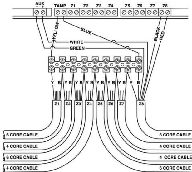
**NOTE** The control panel is supplied with a link fitted across the Global System Tamper to simulate a closed circuit. This link would usually be removed during installation. However the Global System Tamper will typically only be used with normally closed operation, with EOL operation the tamper link would usually be left in place.
