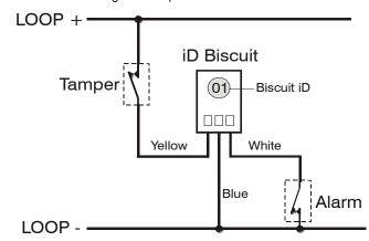
When the tamper switch is opened, the iD biscuit is taken offline and a tamper condition is generated by the control panel. If the alarm switch is opened the biscuit's internal sensor changes state and the control panel will see this as an active condition and will respond as appropriate.
