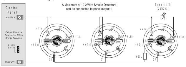
To enable 2-Wire smoke detection on panel output 1, a jumper link must be fitted across the bottom two pins of JP10. The Area Option '2-Wire Smoke' also needs to be enabled (see page 67).
