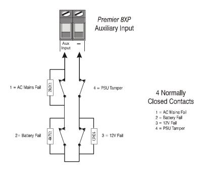
When the Auxiliary Input is programmed as 'PSU Monitor' the system will respond as follows:
