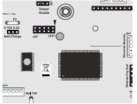
The DTMF chip is located to the left of the main processor and is identified with a green dot.
