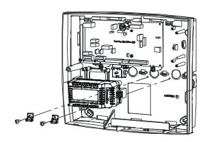
Step 2: Fit battery into place, position the clamps against the top face of the battery and tighten screws.
