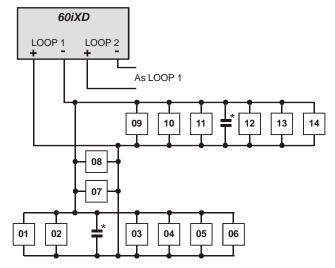
\* The 60iXD expander module is supplied with 4 off 10nF capacitors in the spares pack. It is recommended that you connect a 10nF capacitor approximately at the half way point of each iD spur. It is especially important to do this on iD spurs that are less than 30 metres.
