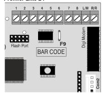
The DTMF chip is located below the Barcode label and is identified with a green dot.
